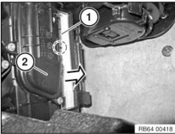
Remove the upper microfilter (1) from the heating and air-conditioning unit (2) in direction of arrow.
