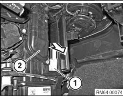
• Remove the lower microfilter (1) from the heating and air-conditioning unit (2) in direction of arrow.
