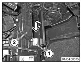
• Install the lower microfilter (1) in the heating and air-conditioning unit (2) in direction of arrow.
