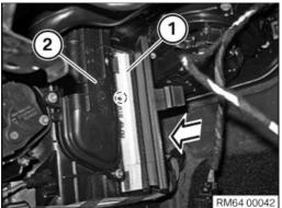
• Install the upper microfilter (1) in the heating and air-conditioning unit (2) in direction of arrow.
