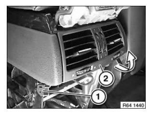
Unclip catches (1) on both sides. Carefully lift out fresh-air grille (2).
