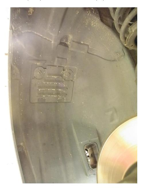
a. There are a total of eleven (11) 8MM-headed bolts and one (1) 10MM plastic nut holding the fender liner. Under the front of the car there are four (4) bolts holding the
