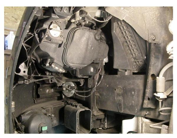
4) **Remove the Halo light holder unit**. Note the polarity of the wires! This is DC power, so you have to keep the polarity correct. The "center" spade is the Green (power) wire; it's covered by a white plastic sheath, the Brown wire (ground) is bare.
