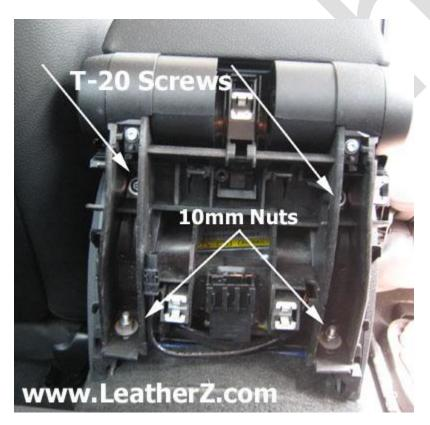
To remove the armrest, you will need to lift it up until it clears the 2 captive bolts at the base. The center console has enough play to allow you to clear the bolts. Once you have the armrest over the two bolts, slide the armrest back.
