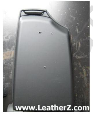
A new armrest will not come with the sleeve. The sleeve is expensive, so you will want to re-use it. To transfer it to a new armrest, use a piece of paper with the paper aligned with the longer (left in the picture above) and the bottom edges. Use a pencil to mark the holes on the paper. Align the paper on the bottom of the new armrest and transfer the holes to the new armrest. The T-20 screws
