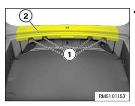
• Secure expanding rivet (1) of the loading edge trim (2).
