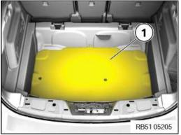
Remove the luggage compartment floor trim panel (1) upwards.
