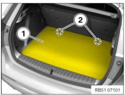
• Raise the luggage compartment removable panel (1) slightly, detach it from the latch mechanisms (2) and remove towards the back.
