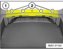
• Unclip the trim of the loading edge (1) at the latch mechanisms (2) in an upward direction and remove.
