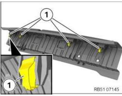
• Check the clamps (1) for damage and renew if necessary.
