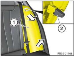
► Removing backrest side section without airbag
