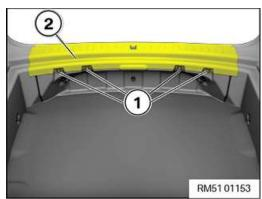
• Open the expanding rivets (1) of the load edge trim (2).
