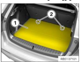
• Clip luggage compartment removable panel (1) into latch mechanisms (2) and set down.
