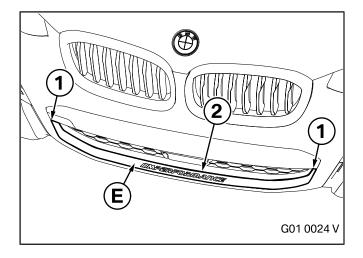
Align the high front gloss black film **E** in the centre, pressing both sides (1) into the corners of the air intake grille and ensuring that the edge (2) runs straight. Press the front gloss black film **E** into position and run the squeegee over it.
