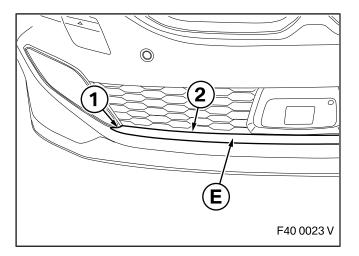
Align the front high gloss black foil application  $\mathbf{E}$  in the centre, pressing both sides (1) into the corners of the air intake grille and ensuring that the edge (2) runs flush along the air intake grille. Press the front high gloss black film  $\mathbf{E}$  into position and run the blade over it.
