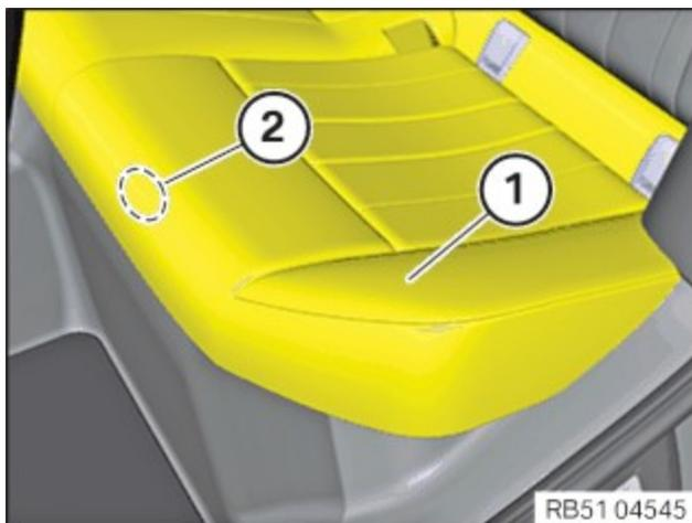
Release rear seat (1) in area (2) in upward direction from the latch mechanisms.
