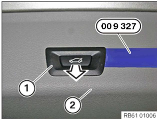
Lever the switch for the tailgate lift (1) out of the tailgate trim panel (2) with the special tool 0 496 571 (00 9 327).
