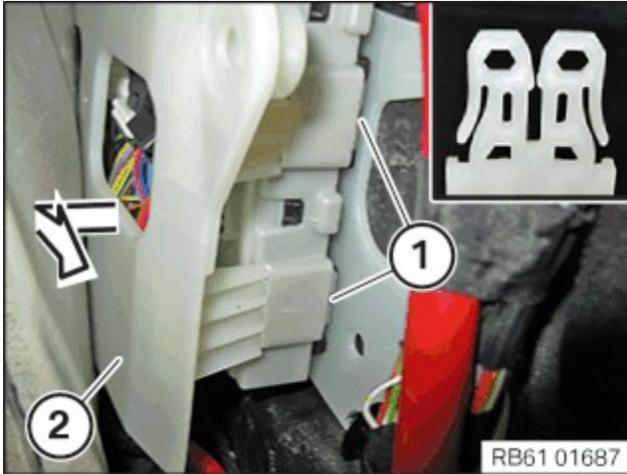
Loosen the latch mechanisms (1).
