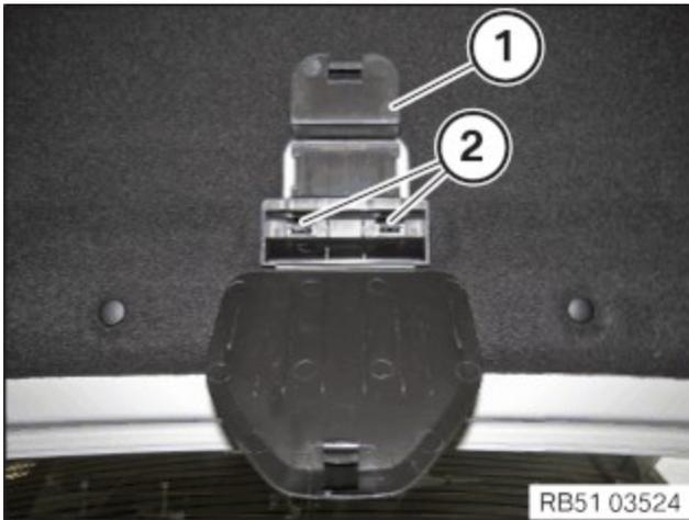
Detach the holders (1) at the latch mechanisms (2) and remove them towards the bottom.
