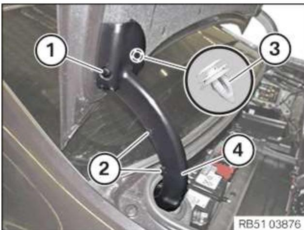
Loosen expanding rivet (1).
