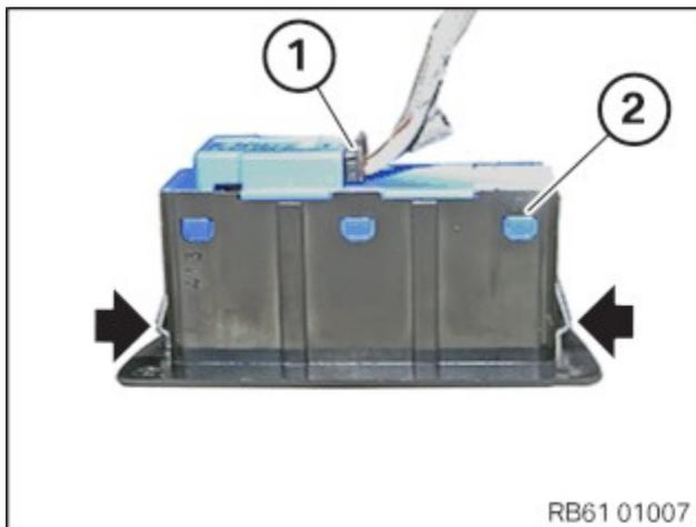
Unlock and disconnect the connector (1) on the switch (2).
