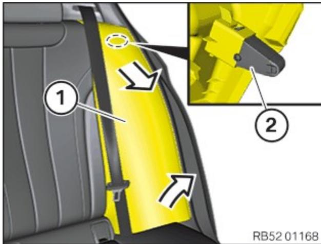
Reach behind the backrest side section (1) from the top and unclip the backrest side section (1) from the latch mechanism (2) to the front.
