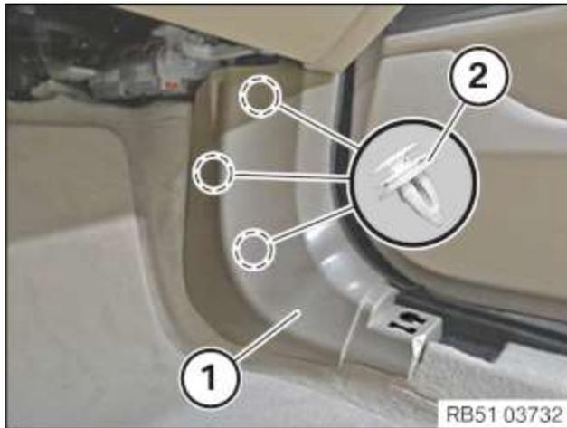
Loosen the side trim panel (1) at the clips (2) and remove it toward the inside.
